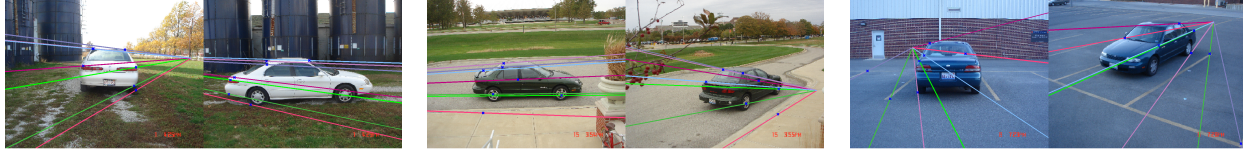
Figure 4. Example ultra-wide baseline matching [36] output. Estimated epipoles and epipolar lines (colors correspond) for image pairs.
